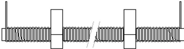
2) Heating elements with round wire coiled on ceramic support.
